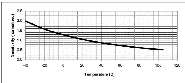
Figure 1: Thermal Accelerometer Sensitivity
