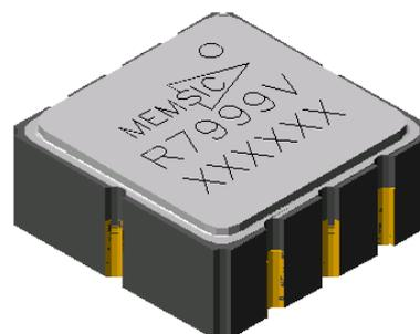
**Note:** The MEMSIC logo's arrow indicates the -X sensing direction of the device.
