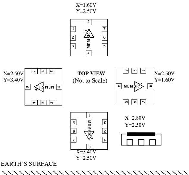
**Note:** The MEMSIC logo's arrow indicates the -X sensing direction of the device. The +Y sensing direction is rotated 90° away from the +X direction. Small circle indicates pin one (1).
