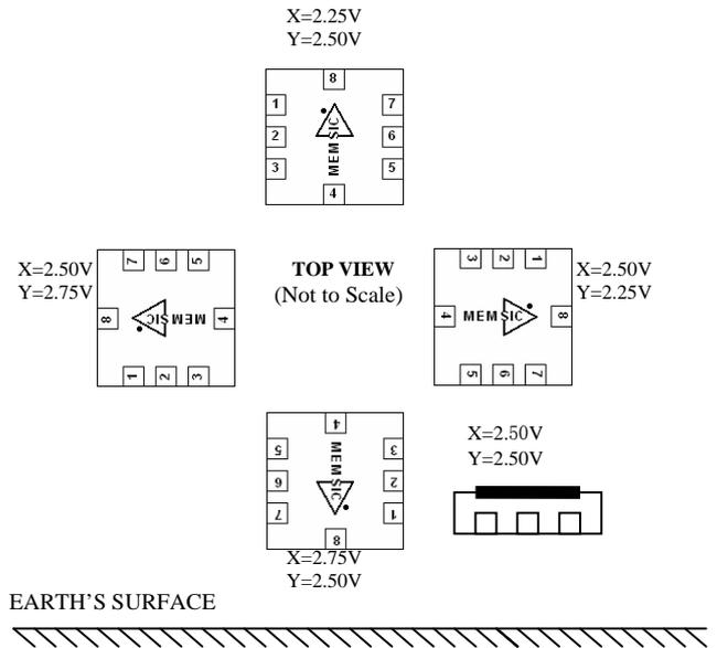
**Note:** The MEMSIC logo's arrow indicates the -X sensing direction of the device.
