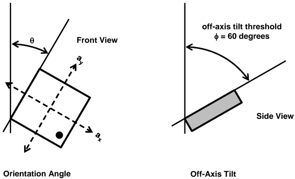
FIGURE 5: Orientation Angle and Off Axis Tilt
