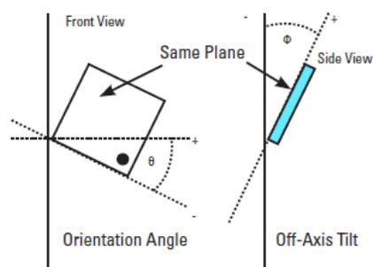
Off-axis tilt is the angle of the x-y plane of the device from vertical (See figure above). As off-axis tilt increases from 0 to 90 degrees, the magnitude of the acceleration vector in the x-y plane decreases. If the acceleration signal is too small, an accurate determination of orientation cannot be made. Angle accuracy is degraded when off-axis tilt angle exceeds  $\pm 15$  degrees. Orientation detection is disabled if off axis tilt exceeds approximately  $\pm 60$  degrees.
