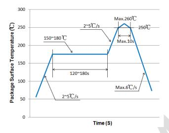
Figure 8: Recommended solder reflow profile
